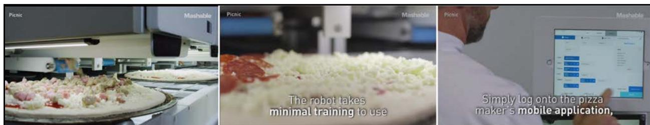
Working near a hot pizza oven must be difficult at times for employees. This machine makes up to 300 twelve inch pizzas per hour, or 180 eighteen inch pizzas per hour. Employees need only fill the ingredient bins periodically, similar to filling ink cartridges for a colour printer. **Picnic**, the maker, claims better uniformity in all orders. [*Pizza vending machines in large cities are able to re-heat frozen pizzas, similar to supermarket freezer products.*]
